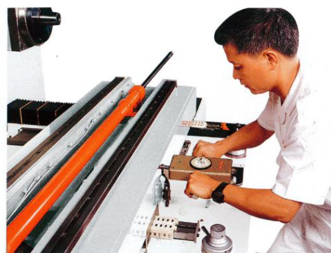
Driving force test on saddle
