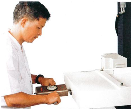
Driving force test on table
